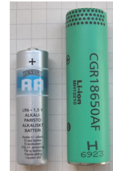
18650 battery, next to a AA battery for comparison
