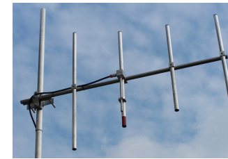
vertical Yagi antenna showing its elements held in place by the boom
