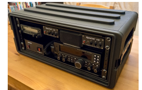
enclosure-mounted HF rig
