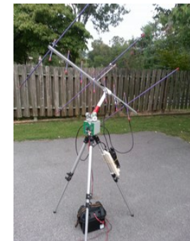
az-el rotator shown on a satellite antenna mount
