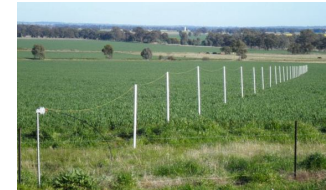
modern 160-meter Beverage antenna, about 280 m in length
