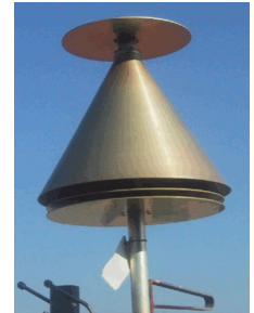
discone antenna of sheet metal
