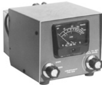
27-17 Amateur radio RF wattmeter.
