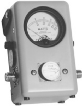
27-18 Bird model 43 RF wattmeter.
