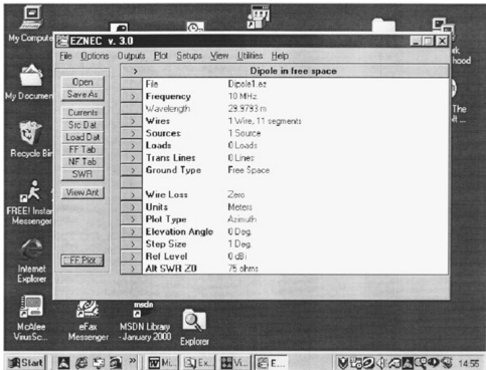
17-8 Basic window of EZNEC for Windows.
