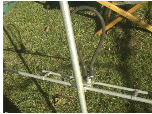
Fig 34 – A Half-Wave Balun
