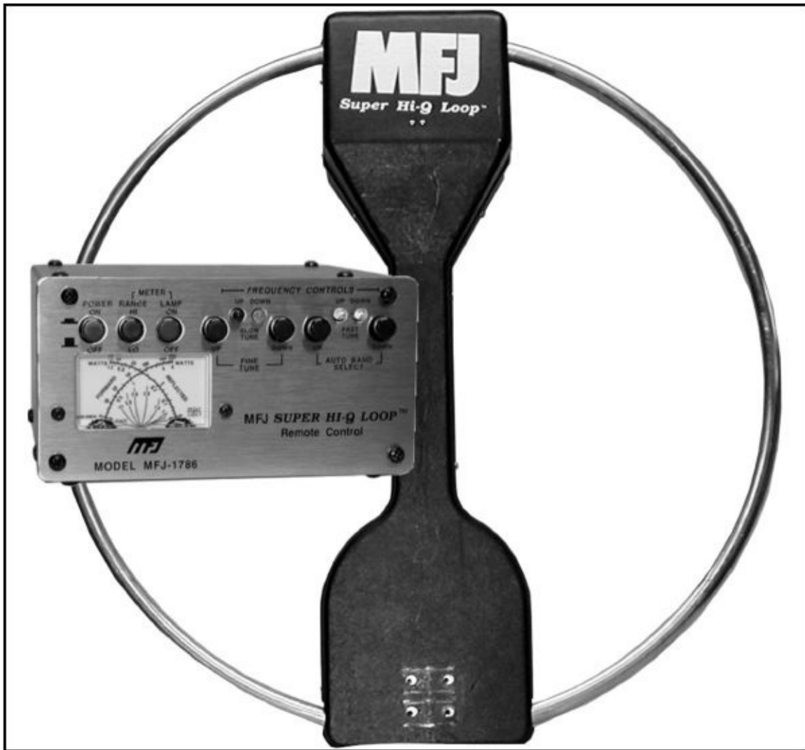
The MFJ-1786 is a small loop antenna with a remotely tuned capacitor to resonate it on 30 through 10 meters.
