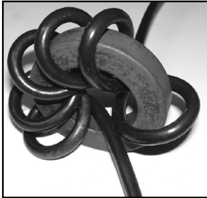
An example of a common-mode choke made by winding coaxial cable through a 2-inch ferrite toroid.
